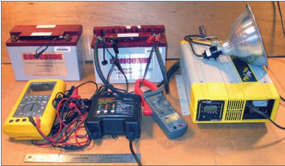
Test set, above, consisted of inverter-based load for discharging and recording volt and ammeters. Temperature probe attaches via a ring terminal, left.
