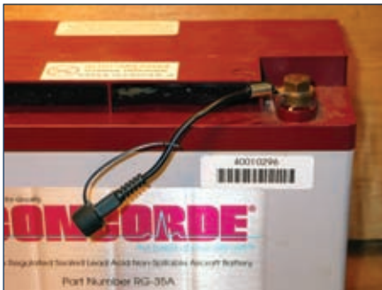
Test set, above, consisted of inverter-based load for discharging and recording volt and ammeters. Temperature probe attaches via a ring terminal, left.
