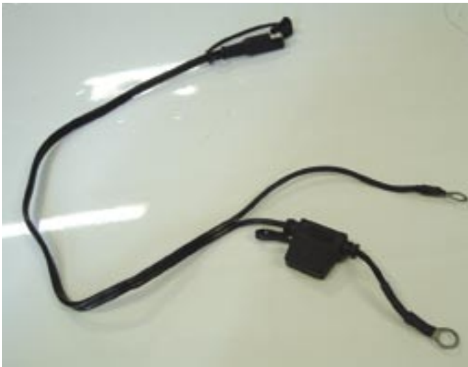
Battery Minder leads in PA-32 forward baggage.
