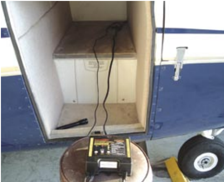
Picture showing Battery Minder hooked up and operating.
