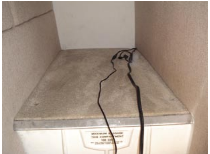
Battery Minder leads connected in baggage compartment.
