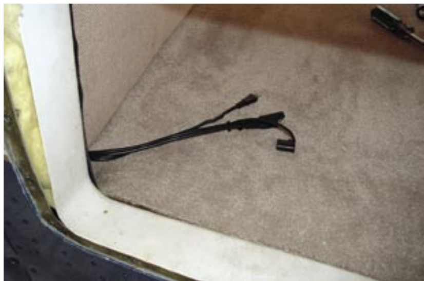
Battery Minder leads extending out of baggage compartment floor.
